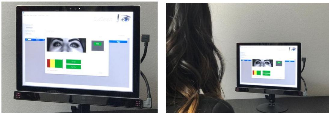
EyeDetect is a hardware and software solution. The hardware is an Intel NUC7i5BNK mini-PC with Windows 10. A high-definition, infrared eye-tracking camera is mounted along the bottom of the monitor. This eye tracker takes 60 measurements per second of each eye with measurements as small as 1/100 of a millimeter.
